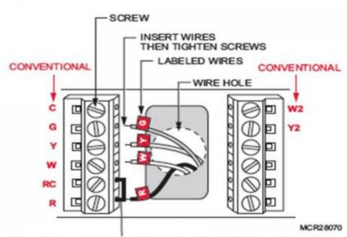
Remove metal jumper if you have both R and Rc wires.
